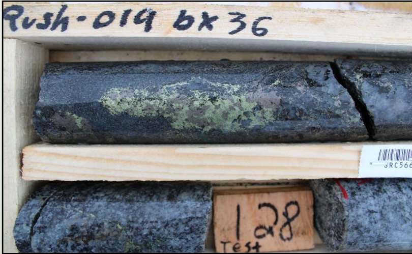
Rush-019: coarse grained chalcopyrite and pyrrhotite mineralization from 127.18-127.38m
