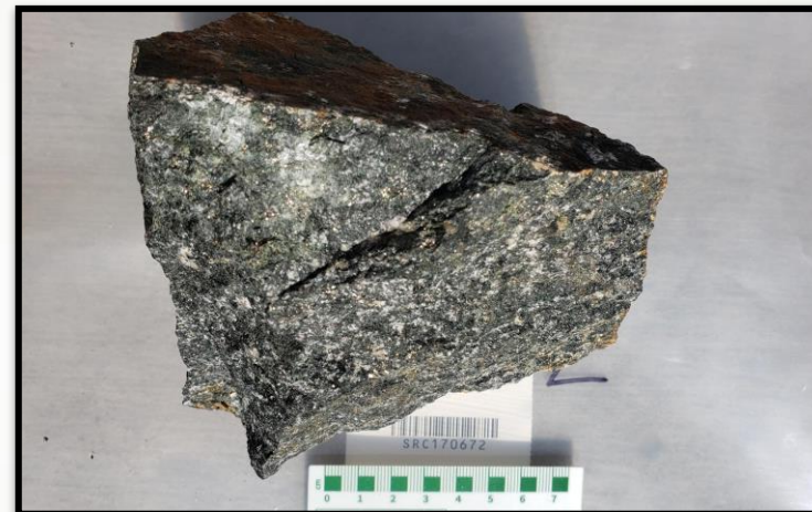
Sample 170672: 1210ppm Cu, 333ppm Ni, 79ppm Co
