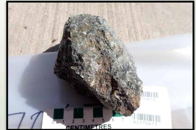
Sample 170673: 1550ppm Cu, 451ppm Ni, 104ppm Co
